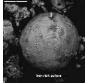
Iron-rich spheroid from the USGS Particle Atlas of World Trade Center Dust. 960 This 20 \mu\text{m} diameter sphere is comparable to ones found in the Crop Circle Soil Samples
